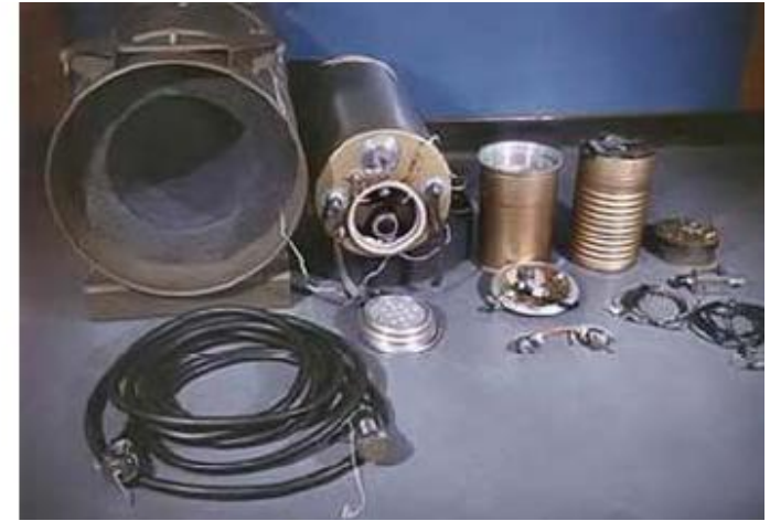
Medium Atomic Demolition Munitions (MADM) – Fully Assembled (left) and Unassembled (right). Assembled package weighs ~400 pounds – Yield = 1-15 kilotons ; according to http://en.wikipedia.org/wiki/Medium Atomic Demolition Munition
